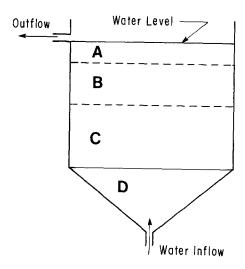
Figure 1. Scale drawing of the depth sections in the Tank Position Experiment. Tank diameter is 20 cm.
